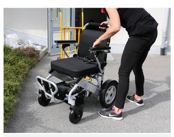
3 Unfold the Eloflex by pulling the backrest up and back. Lock the hook under the backrest (see the instruction manual).
