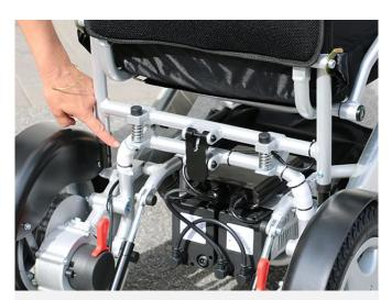
Remove the protective packaging material on the rear arch above the motors by cutting the zip-ties.
