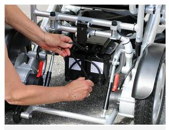
Plug the loose cable into any available outlet on the battery. Tighten the locking ring firmly around the outlet.
