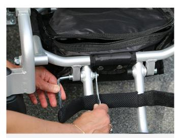
12 The inertia of the footrest can easily be adjusted by tightening or releasing the two fixing screws. You can then lock the nut with loctite (see picture).
