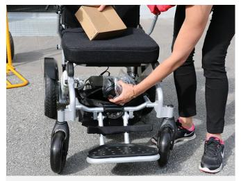
7 Take out the joystick from the bag underneath the seat.
