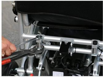
11 If the locking hook feels stiff and difficult to open/close, it can be adjusted by tightening the two springs (see picture).
