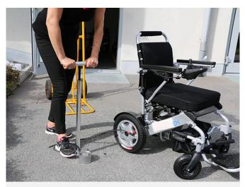
**10** Pump the rear wheels of the F and P to 2,5 kg air pressure
