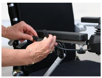
**9** Carefully assemble the contacts on the joystick cable after checking the guiding tracks. Do not bend the pins! Tighten the locking rings.
