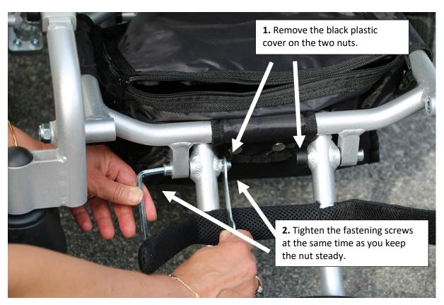
**Tip**: Lock the nuts with loctite after you've adjusted them, so you don't have to redo the process in the future.
