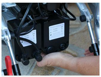
3 Place your hand under the battery and try to find the clamp (see picture 5). Squeeze and gently pull the battery out.
