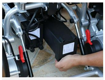
**4** Continue to pull the battery outward until it fully detaches from the holder. Store the battery cautiously.
