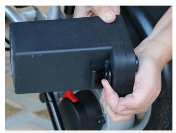
On the underside of the battery there is a clamp that holds it in place in its holder. To release the battery, the clamp must be pressed.
