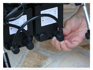
1 Unscrew the locking ring on the bottom of the battery until it's completely loose.
