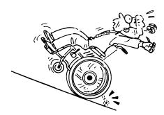
Be careful when driving on steep slopes, as the chair is likely to break. Eloflex is tested and approved for gradient with a maximum of 9 degrees.
