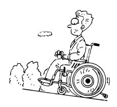
• Driving on slopes. Try driving straight up or down for an inclined surface. Lean slightly forward as you drive up, and backwards as you drive down, to maintain the center of gravity. Avoid driving sideways if possible and compensate for any side slope by leaning in the opposite direction. Always drive slowly on slopes. Avoid surfaces that tilt more than 9 degrees.
