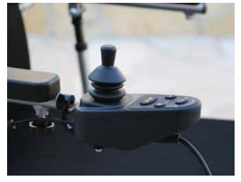
should take place for about five hours when the bar on the battery indicator at the joystick has dropped to one third (when three of the lights are green). The batteries will not be damaged by maintenance charges but for maximum battery lifespan we recommend that you disconnect the charger when the batteries are fully charged.
