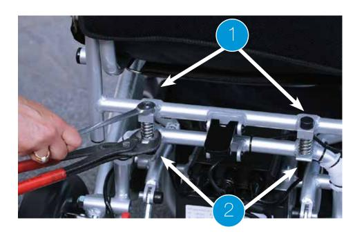
It is important that the lock on your Eloflex is tight to pull up and down. It should go so slowly that it can stand straight out by itself as in the picture above. This is important for the lock to stay in its locked position even if the springs are pressed together. To make the lock more tight, you just need to tighten the bracket with the two hex screws that hold the lock in place.
