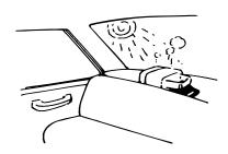
Never leave your Eloflex in direct sunlight or near a heat source as the batteries may be damaged. Never be near open fire with your Eloflex.
